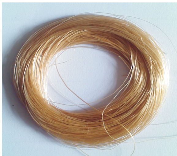
Figure 1. Gelatin-PEG-MMT nanocomposite fibers prepared by gel-spinning. [Color figure can be viewed in the online issue, which is available at wileyonlinelibrary.com .]
